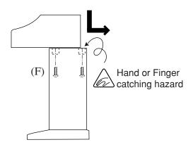
3. Place the piano on the front half of the stand so that the metal fitting holes are seen when viewed from the top. Slide the piano backward while holding it with one hand so that it does not incline and fall from the stand. The hooks on the piano are then engaged with the metal fittings on the Side Panels. Pay attention so that your hand or fingers are not caught between the stand and piano. Fasten the piano and the stand with four bolts (F).
